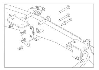
21. Under the tub, Drill 2x 3mm pilot holes at the slots center of the RHS rear mounting bracket.
