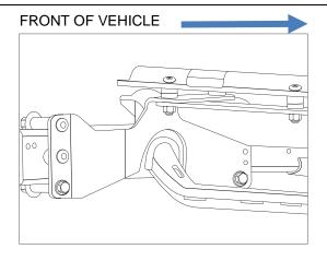
39. Place a spacer between the LHS Rear mounting bracket and brake lining bracket. Secure the brake lining bracket with a supplied M8 bolt. Refit the brake lining plastic clip, the rubber tube clip and the harness clips.
