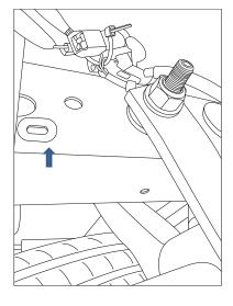
Remove 1x M8 bolts on the brake line bracket and 1x fir tree clip from the chassis. Remove 4x harness fir tree clips from the chassis.
