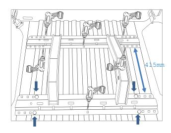
26. Check the pilot holes are near the slots center of the LHS – RHS front mounting brackets.
